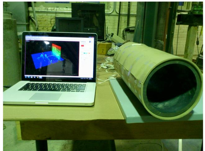
Figure 7 Instrumented Pipe with Protective Layers
