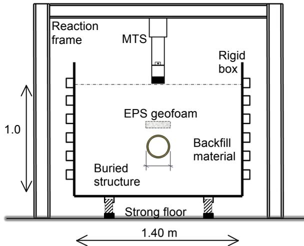
Figure 8 Schematic of the Test Setup
