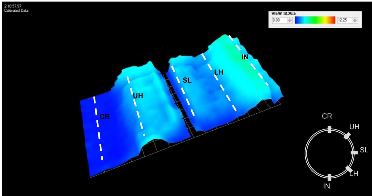
Figure 12 Snapshot of the Earth Pressures around the Pipe after Geofoam Installation
