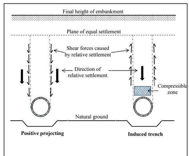
Figure 1 Positive Projecting versus Induced Trenching
