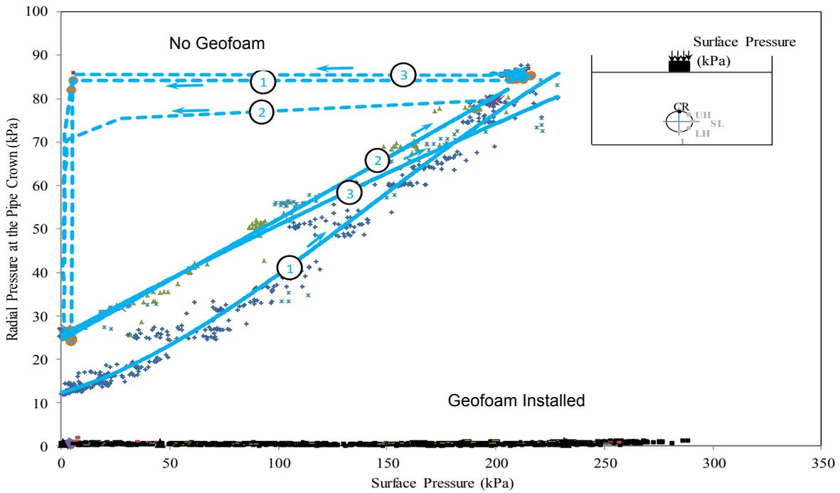
Figure 14 Earth Pressures in Cyclic Loading (Crown)
