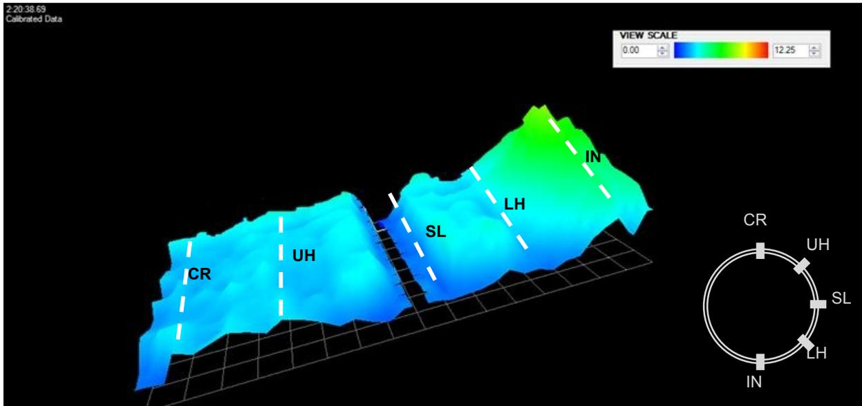
Figure 11 Initial Earth Pressure Distribution (Without Geofoam)
