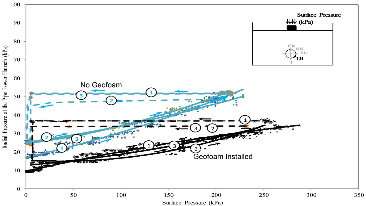
Figure 15 Earth Pressures in Cyclic Loading (Lower Haunch)
