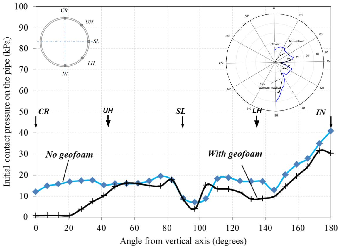
Figure 13 Initial Earth Pressure Distribution on the Pipe
