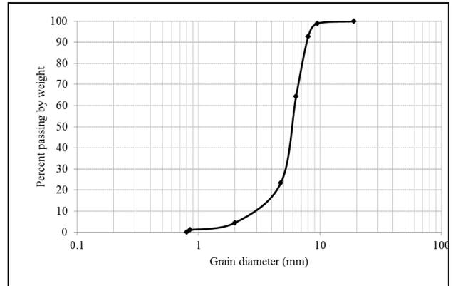
Figure 6 Particle Size Distribution of the Backfill Material
